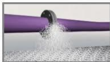
Unprotected leaking flange
