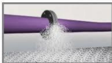
Unprotected leaking flange
