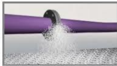
Unprotected leaking flange
